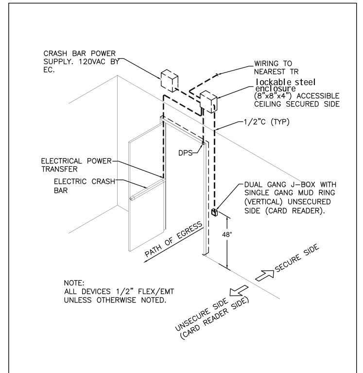
DETAIL: ELECTRIFIED LATCH RETRACTED DOOR (SINGLE)
